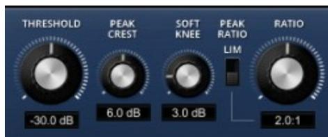
**Threshold** defines the level above the compressor begins to compress the signal. The lower the threshold, the deeper the “grab”.
