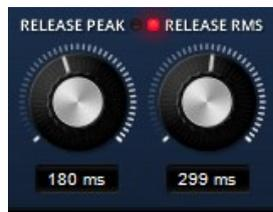
The timing section differs slightly from the typical layout found on most compressors. The TDR Feedback Compressor can dynamically select the most suitable release “path” depending on the program material. Two LEDs indicate the currently active release path and controls.
