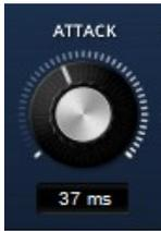
Attack time controls the speed of gain reduction, i.e. how long the compressor takes to reach full gain reduction. Fast attack times quickly respond to level changes in the side-chain. Slow attack times on the other hand respond smoothly and let small event pass through the compressor without reduction.
