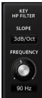
The Key High-Pass Filter section allows to control the compressors sensitivity for low frequencies. That is, the compression threshold becomes frequency dependent and thus less responsive to low frequency content. Three different high pass filter slopes are supported:
