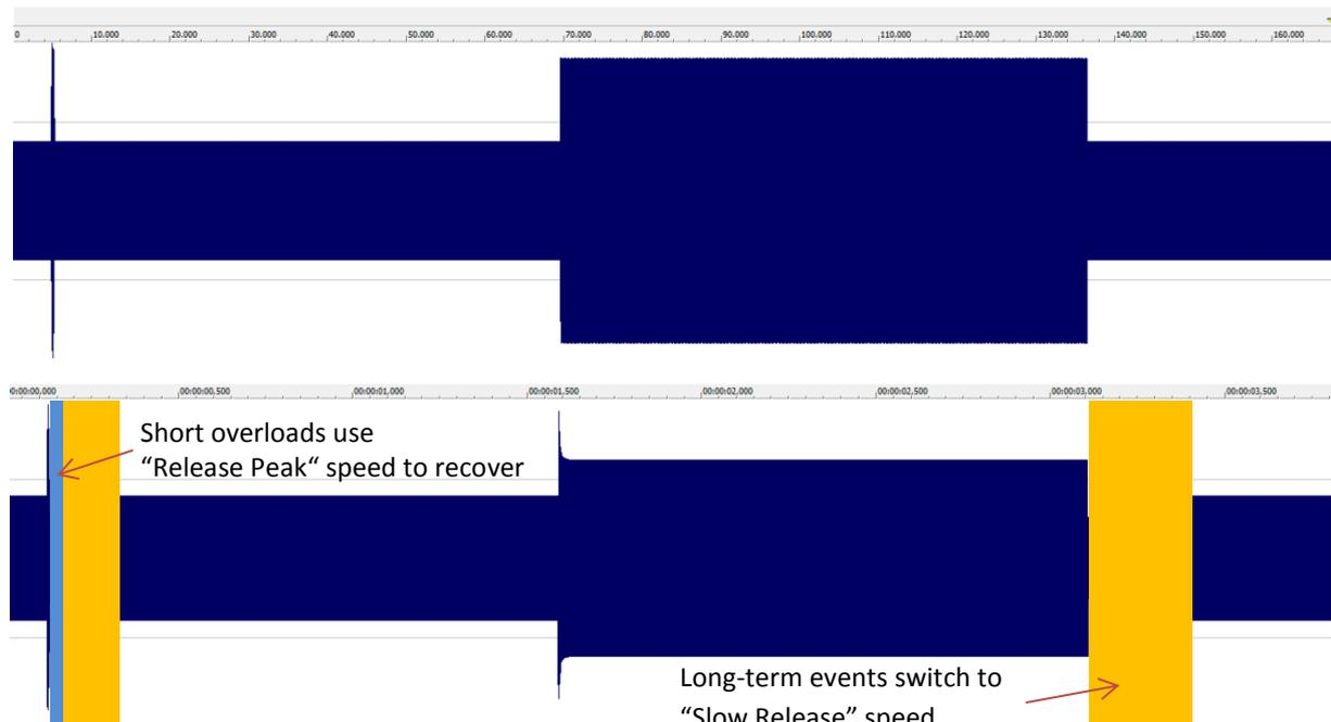
Two release paths offer a wide range of musically useful options. For example, single drum peaks can be allowed to recover quickly to avoid “dulling” and “breathing” side-effects. At the same time, sustained content like bass-lines or synth pads can recover slower and thus strongly reduce typical side-effects like “pumping” and distortion.
