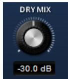
**Dry Mix** blends the original signal into the processed (i.e. compressed) part. It enables the use of parallel compression techniques (upward compression, “NY compression”) without the complicated routings and latency compensation inside the DAW.
