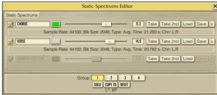
Some Voxengo equalizer plug-ins feature static spectrums display that can be controlled via the editor window shown above. You may select the display name of the spectrum slot, its color, the shift in decibel of the static spectrum on the control surface. The static spectrum can be shown or hidden via the visibility check box.
