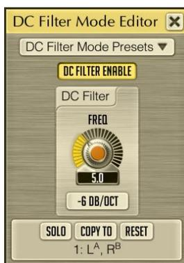
This window allows you to fine-tune the DC filter, and create user presets if required. DC filter (also known as high-pass filter) is applied after all processing stages, and is used for removing ultra low-frequency content introduced by plug-in’s processing modules.
